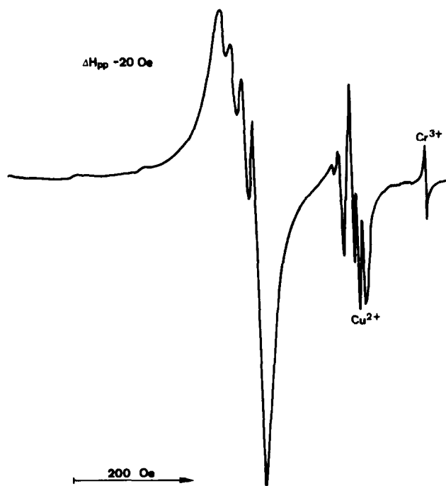
FIG. 5. ESR spectrum of 0.05% Cu-MgO solid solution evacuated for 10 hr at 1200 K. 77 K, gain = 8.0 \times 10^3 , modulation amplitude = 1 Oe.
